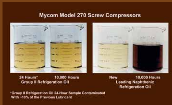
Figure 5. Ammonia Refrigeration Oil Field Demonstration
